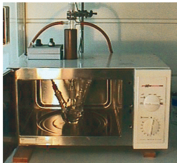
FIGURE 13. Modified microwave oven for emulsion and micro-emulsion polymerization.
